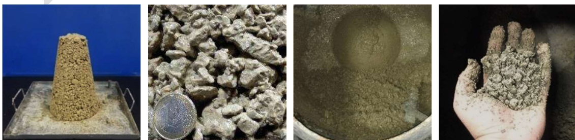
Figure 13. Test specimen exhibiting unstable low slump behavior
