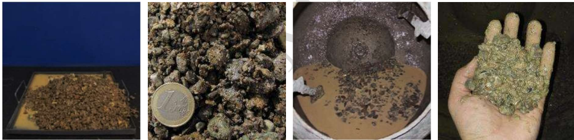
Figure 4. Two distinct phases of diluted liquid and solid grains in the conditioned mix
