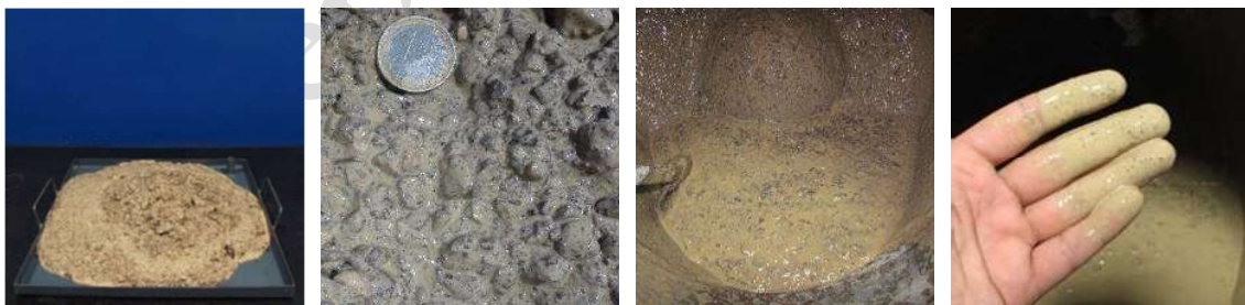
Figure 5. Semi uniform non plastic state of the conditioned mix
