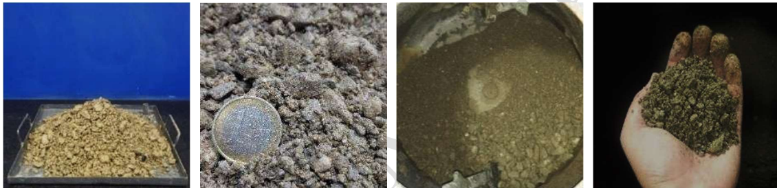
Figure 11. Test specimen in the dampen loose state
