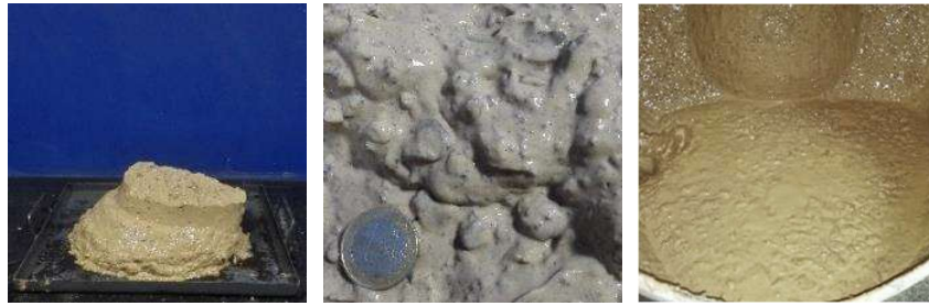
Figure 14. Conditioned material in the over conditioned state
