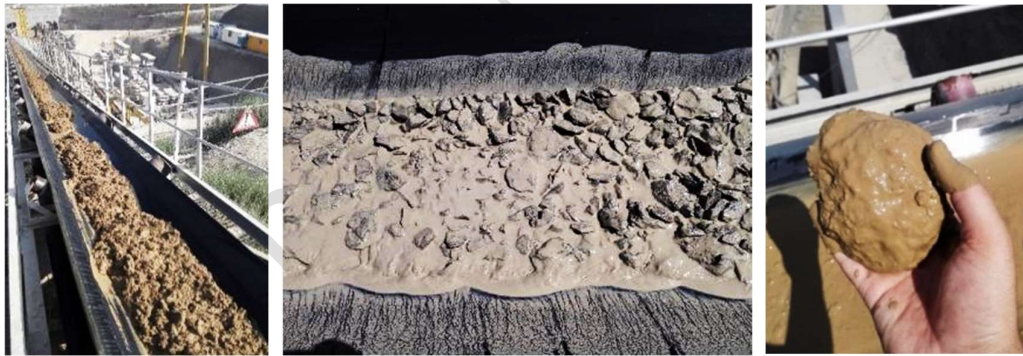
Figure 17. Images depicting well-conditioned material (left), Distinct phases of thin suspension and solid (middle), and formation of bentonite clumps (right)
