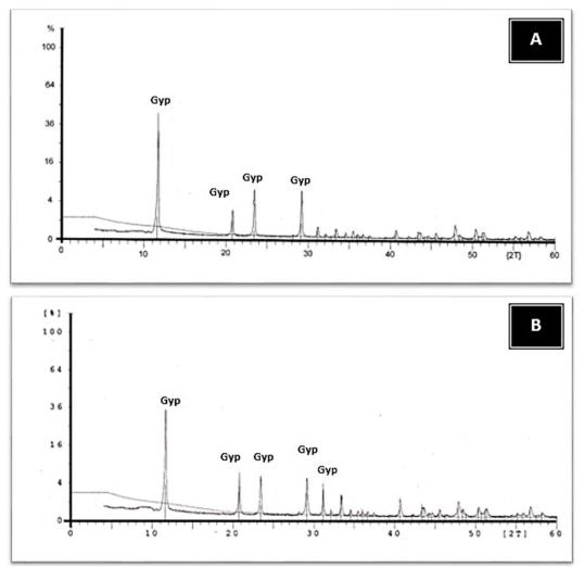
**Figure 4.** XRD analysis of the evaporate samples of the Pesteliegh Formation in the Chehelkaman section. A: XRD analysis of the evaporate samples from the lower parts of the Chehelkaman section. B: XRD analysis of the evaporate samples from the upper parts of the Chehelkaman section
