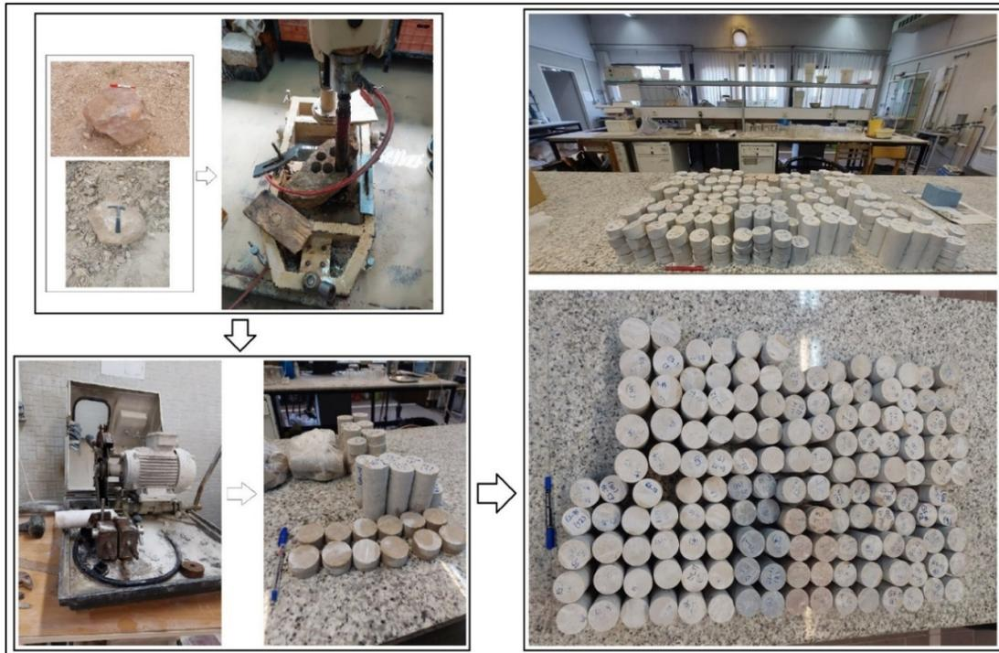
**Figure 3.** Preparing samples for testing
