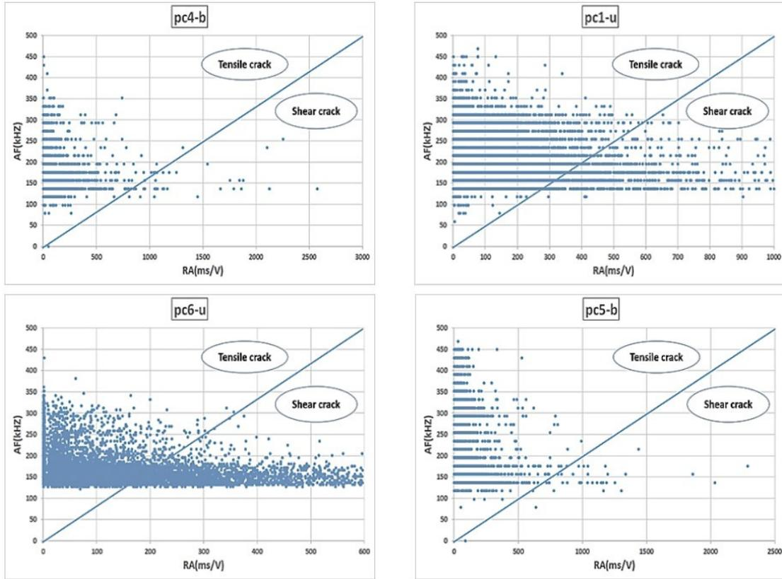
**Figure 2.** Cracks classification in tensile splitting (pc5-b, pc4-b) and uniaxial (pc6-u, pc1-u) tests
