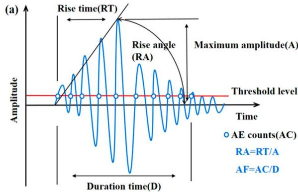
Figure 6. Typical AE waveform and AE parameter in a hit (Aggelis 2011)
