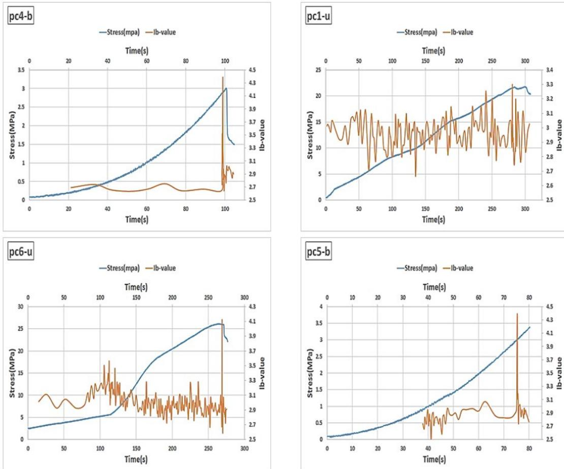
**Figure 12.** Ib-value changes chart and the loading stress for uniaxial test (pc6-u, pc1-u) and tensile splitting test (pc5-b, pc4-b)
