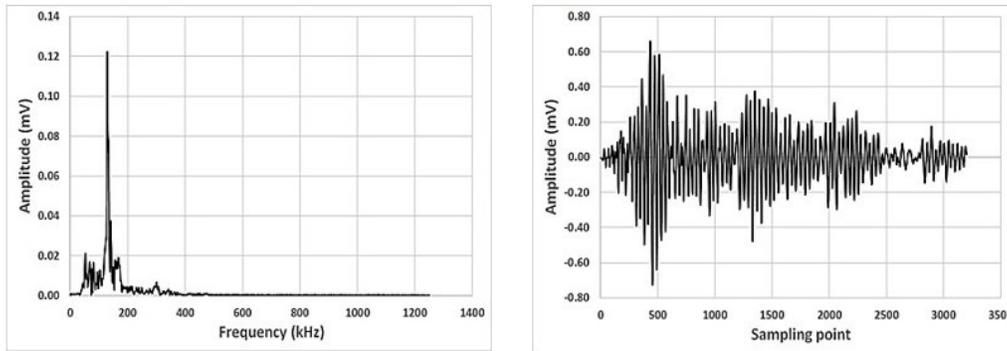
**Figure 3.** AE waveform and the signal frequency spectrum related to uniaxial compressive tests
