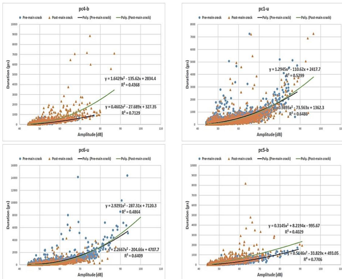
**Figure 14.** AE amplitude distribution versus time duration in uniaxial (pc6-u, pc1-u) and tensile splitting (pc5-b, pc4-b) tests
