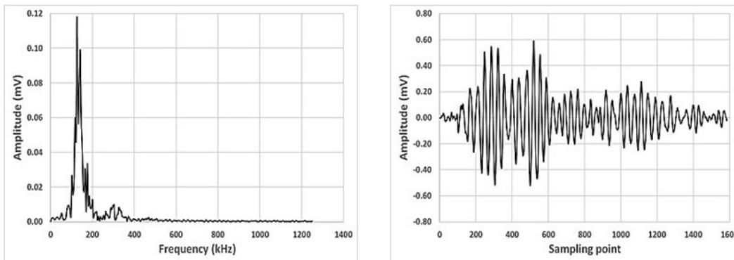
**Figure 4.** AE wave form and signal frequency spectrum related to tensile splitting tests
