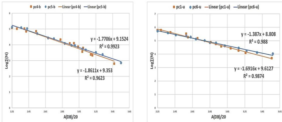
**Figure 31.** b-values in uniaxial (pc6-u, pc1-u) and tensile splitting (pc5-b, pc4-b) tests
