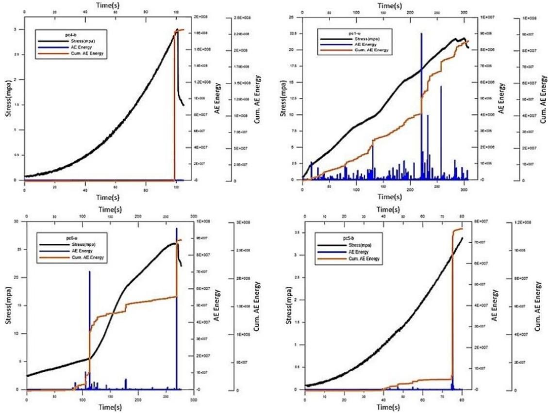
**Figure 5.** The chart of the changes in energy level, cumulative energy, and stress in tensile splitting (pc5-b, pc4-b) and uniaxial tests (pc6-u, pc1-u)
