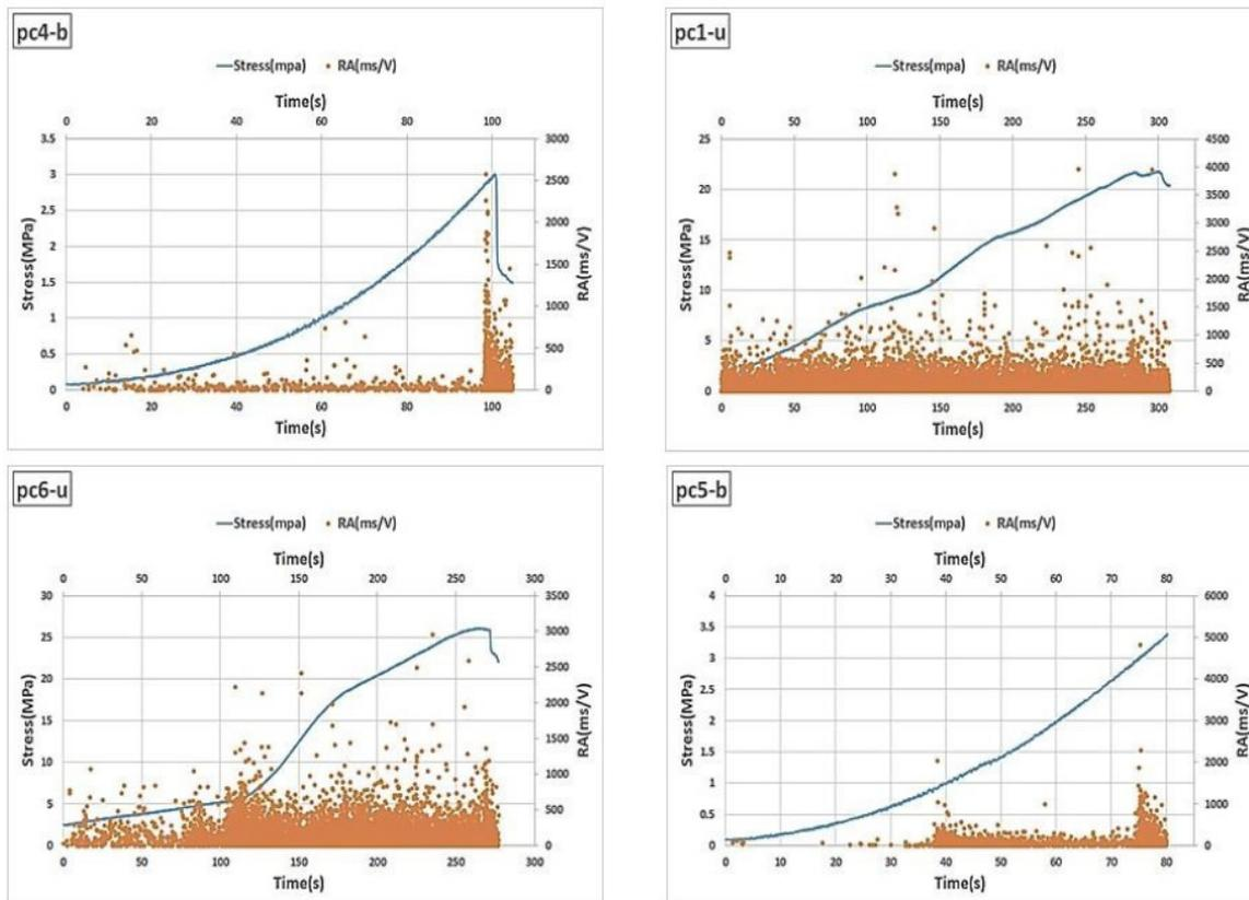
**Figure 8.** Chart of the changes of rise angle and loading stress in tensile splitting (pc5-b, pc4-b) and uniaxial (pc6-u, pc1-u) tests
