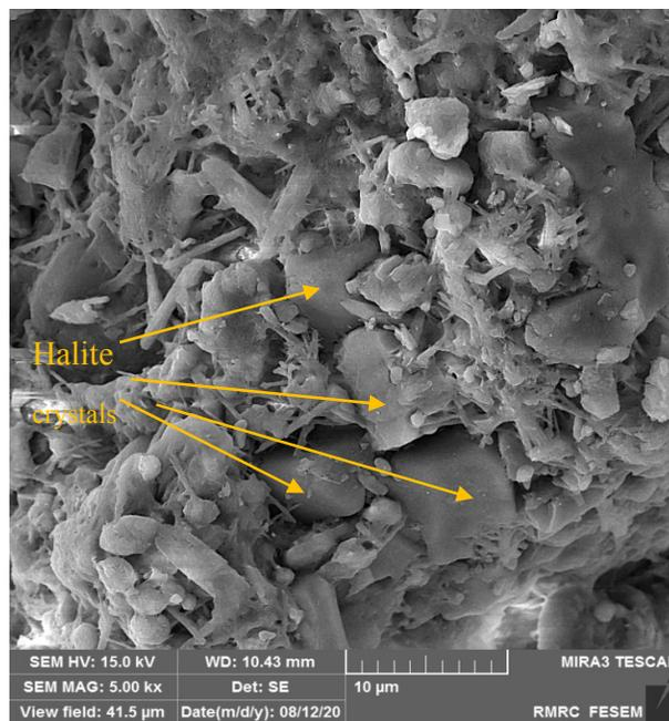
**Figure 10.** FESEM image of Halite crystallization in pore spaces after stabilization with the PGW
