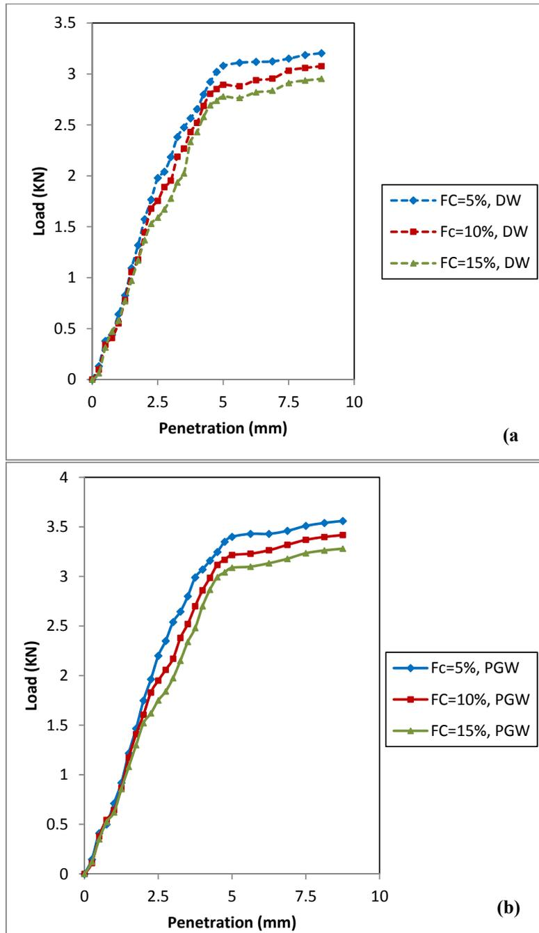
**Figure 8. a)** Variation of the applied load versus penetration value for the samples mixed with DW **b)** Variation of the applied load versus penetration value for the samples mixed with the PGW
