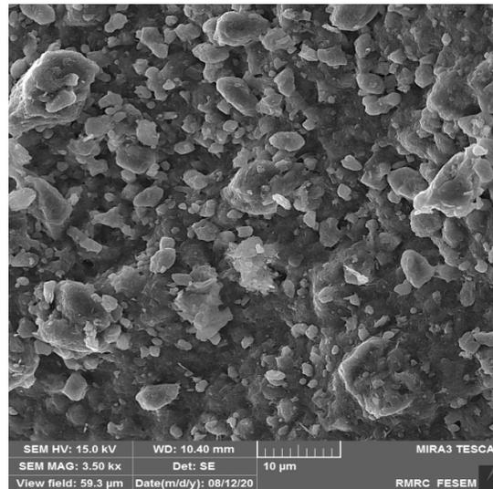
**Figure 4.** FESEM image of SP-SM sample after mixing with the PGW
