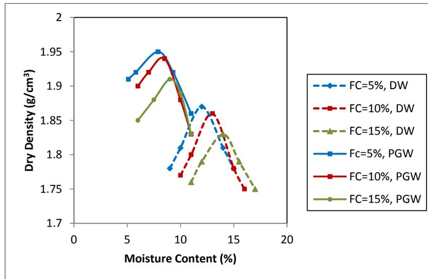
Figure 5. Variation of dry density with moisture content
