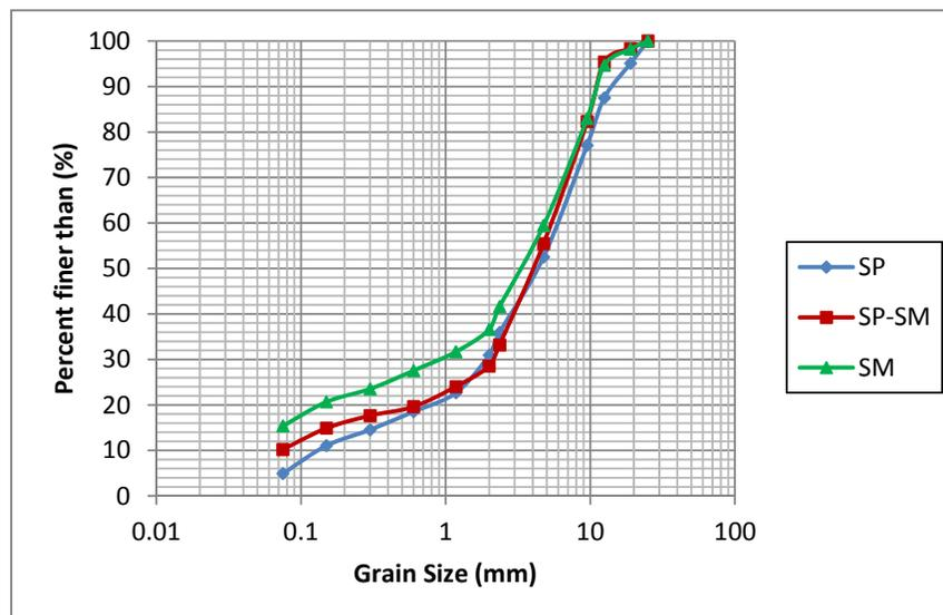
**Figure 1.** The particle distribution curves of the soil samples
