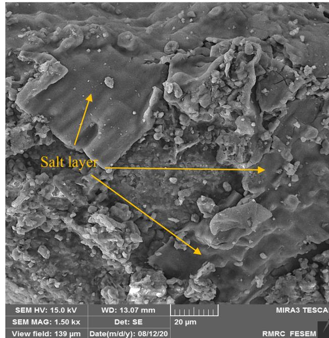
**Figure 11.** FESEM image of the deposition of salt layer on the particle surfaces after stabilization with the PGW
