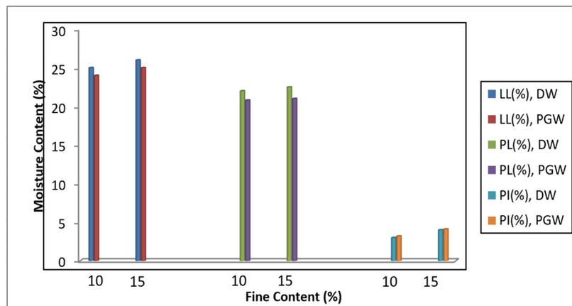
**Figure 2.** Variation of LL, PL, and PI with type of water and fine content percent
