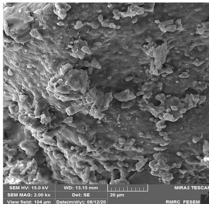
**Figure 12.** FESEM image of surface roughness of soil particles after stabilization with the PGW
