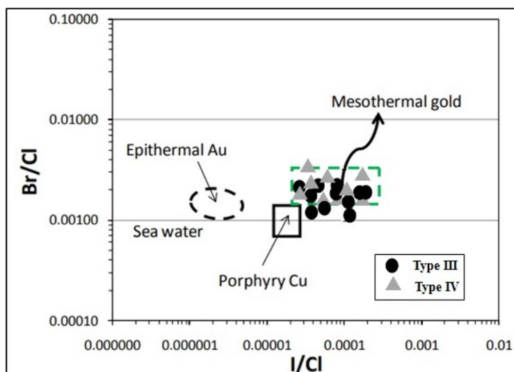
**Figure 12.** Crush-leach analysis of halogen content (I/Cl and Br/Cl ratios) in fluid inclusion showing mineralizing fluids are not identical to magmatic fluid, epithermal (meteoric water-dominated) and porphyry Cu, but tends to be similar to fluids in mesothermal-type (or orogenic) gold deposits
