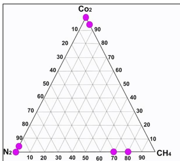
**Figure 11.** Ternary plot of three gaseous components such as  $CO_2$  (98-100 mol %),  $CH_4$  (92-100 mol %), and  $N_2$  (70-80 mol %) in the Lakhshak gold-antimony deposit
