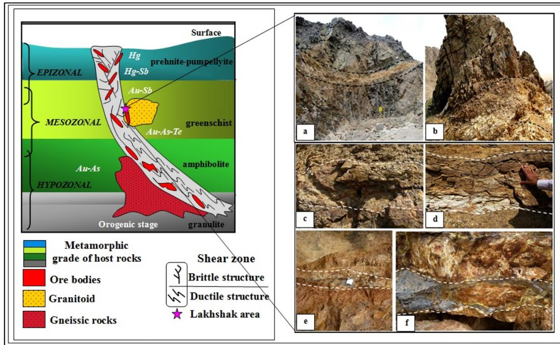
**Figure 13.** The Lakhshak metamorphic-hosted gold deposit plotted on the conceptual orogenic gold deposit model from Groves and Goldfarb (2003) and Groves et al. (2005) emplaced into shallow level at the transition between epizonal and mesozonal (approximately 5-10 km depth below paleosurface)
