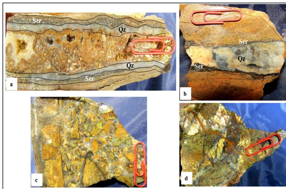
**Figure 6.** (a) Hand specimen of first quartz veins/veinlets parallel to the calc-schist foliation, (b) hand specimen of second quartz vein type crosscuts the first generation of veins as well as the foliation
