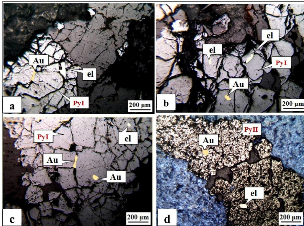
**Figure 8.** Fotomicrograph of free gold (Au) and (el) electrum in quartz vein, inclusion, and vein/veinlets in pyrite
