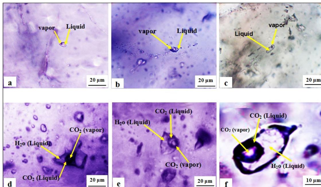
**Figure 9.** Petrographic images of FI types (a, b, c) two-phase (L-V) (Type III), (d, e, f) L<sub>1</sub>-L<sub>2</sub>-V (CO<sub>2</sub>)-rich phases (Type IV) fluid inclusions
