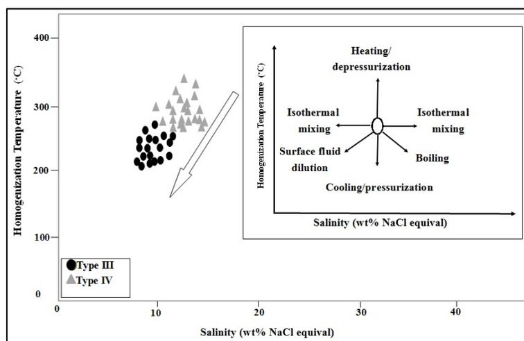
**Figure 10.** Temperature of homogenization ( $T_h$ ) vs salinity of fluid inclusions from quartz veins/veinlets at Lakhshak metamorphic-hosted gold deposit (Wilkinson, 2001). The hydrothermal fluid evolution of these veins/veinlets are also shown and discussed in the text. Schematic model of fluid evolution is adapted from Shepherd et al. (1985)
