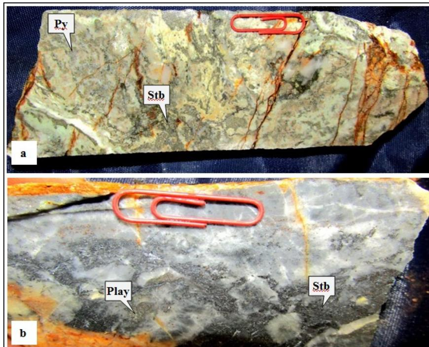
**Figure 7.** (a, b) Diagnostic sulfides (stibnite and pyrite) associated with Lakhshak orogenic gold mineralization. (Stb: stibnite; Py: pyrite) (Abbreviations are given from the Whitney and Evans, 2010)
