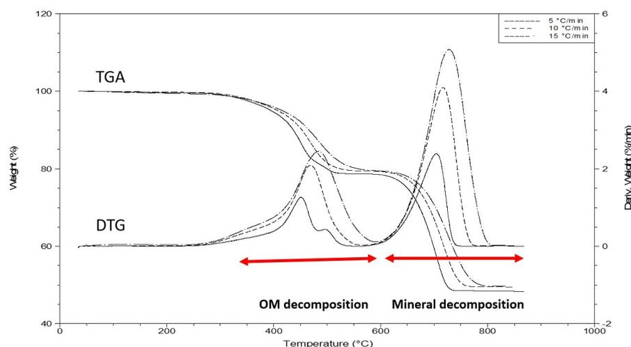
Figure 1. TGA-DTG curves of the representative sample from the Garau oil shale in relation to temperature.
