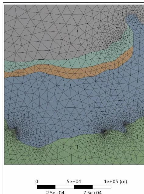
**Figure 4.** Model mesh with ~3626 contact elements and ~7842 mid-nodes
