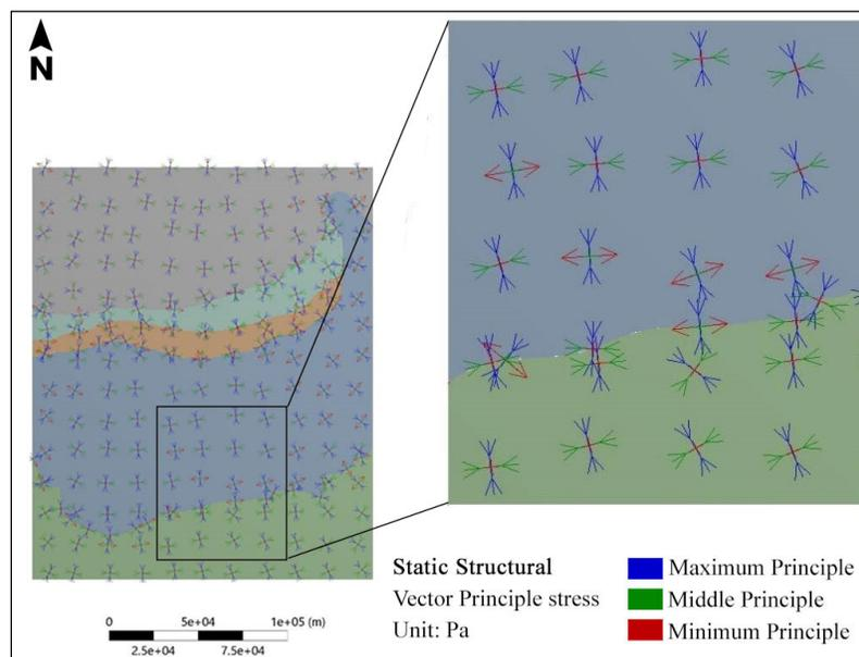
**Figure 14.** Central part of model showing stress patterns along SRT
