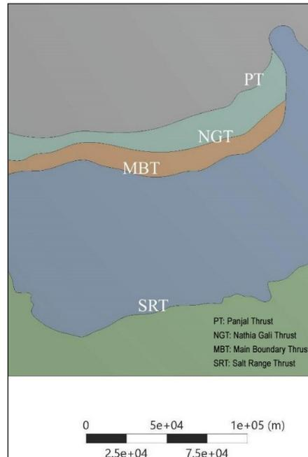
**Figure 3.** Geometry of study area showing major thrusts including PT (Panjal Thrust), NGT (Nathia Gali Thrust), MBT (Main Boundary Thrust) and SRT (Salt Range Thrust).
