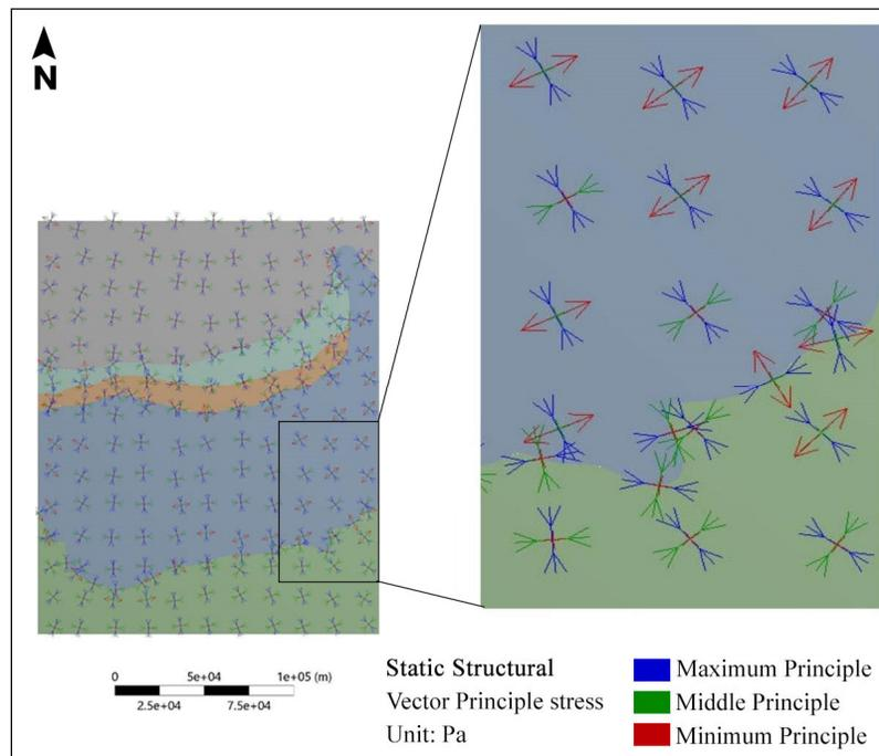
**Figure 13.** Eastern side of model showing stress pattern along SRT
