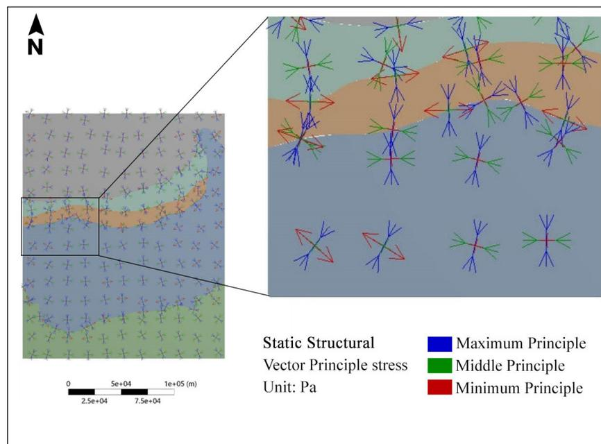
**Figure 12.** Western part of model showing the stress patterns along NGT and MBT
