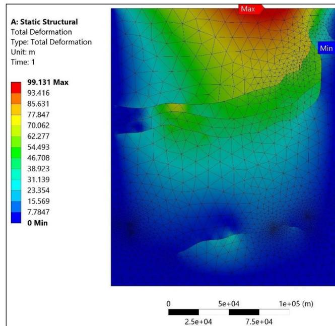
**Figure 15.** Shows total deformation of material under frictional contacts
