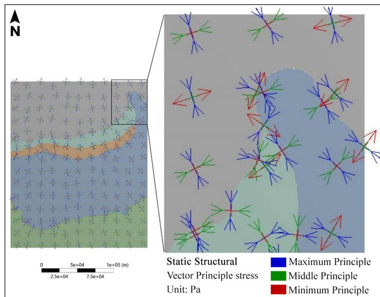
**Figure 7.** Eastern part of model shows stress patterns along Hazara Kashmir Syntaxis and Panjal Thrust
