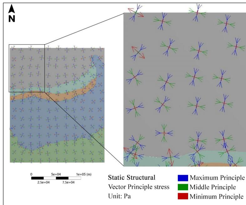
**Figure 9.** Western part of the model shows stress patterns along Panjal Thrust
