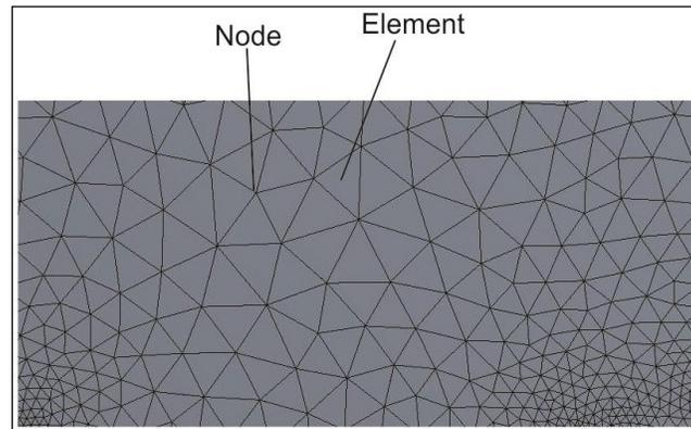
**Figure 2.** Basic triangular meshing in FEM model
