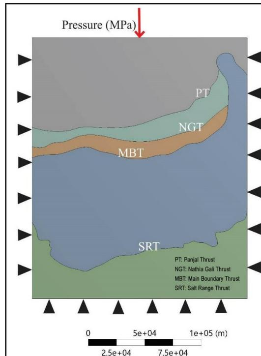
**Figure 5.** Geometry and boundary conditions used in FEM model. Top edge of model is subjected to load i.e., pressure (MPa) from north direction. Black triangles represent the fixed boundary edges
