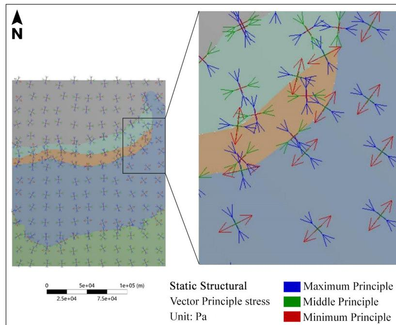
**Figure 10.** Eastern part of model showing stress patterns along NGT and MBT
