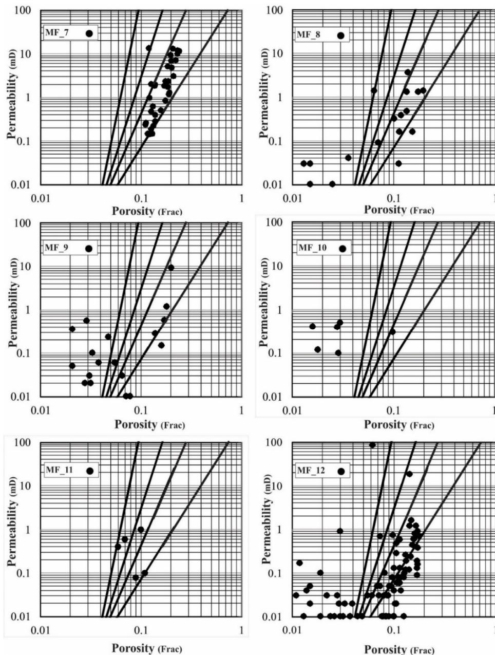
**Figure 13.** Porosity versus permeability on the Lucia rock fabric class Lucia, (2007) for the identified MF7 to MF12
