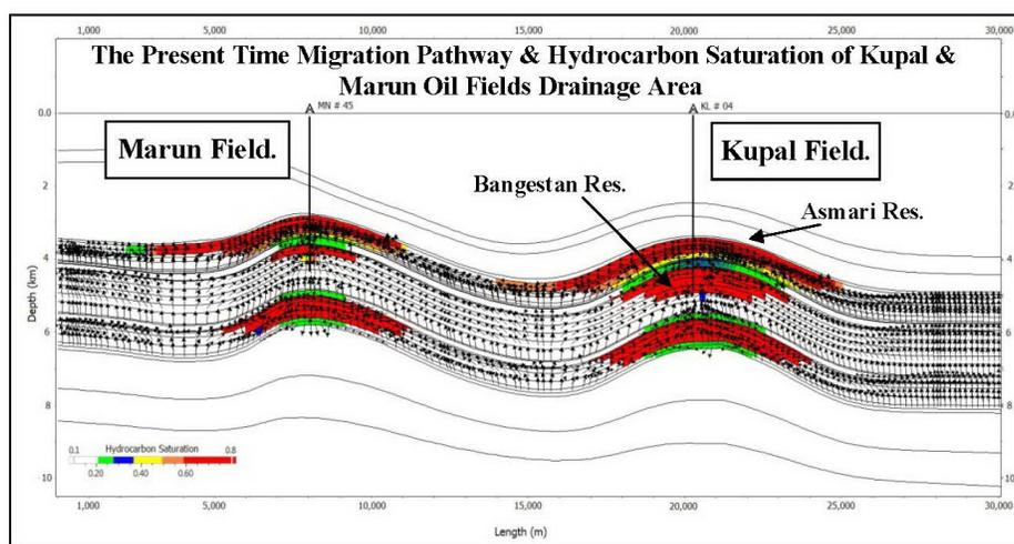
Figure 17. Display of the migration Pathways and locations of accumulated hydrocarbons in the drainage area of the Kupal and Marun fields at the present day.
