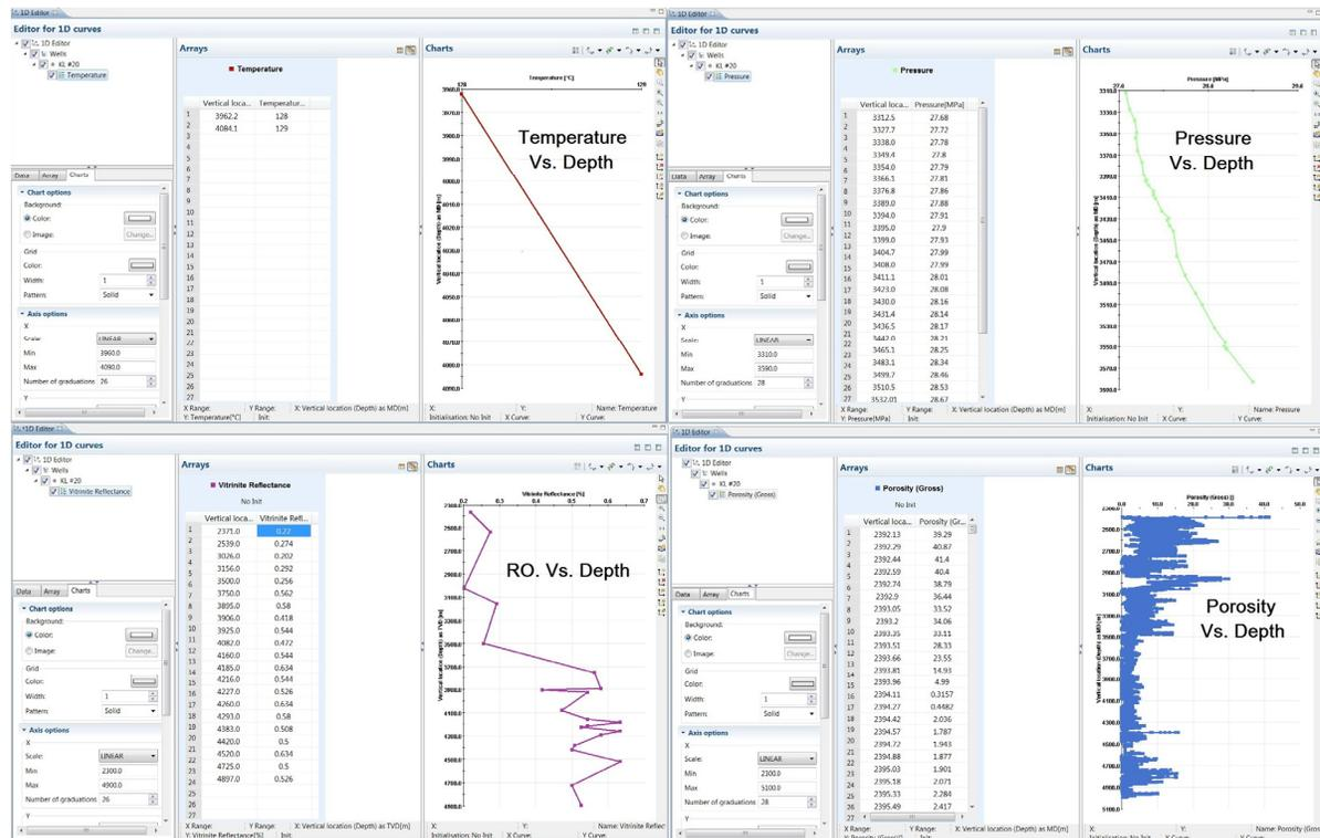
Figure 16. Display of Temperature, Pressure, Porosity and Ro. parameters versus depth to calibrate the Middle Cretaceous – Lower Miocene 3D petroleum system of the Kupal field, well No. 20.
