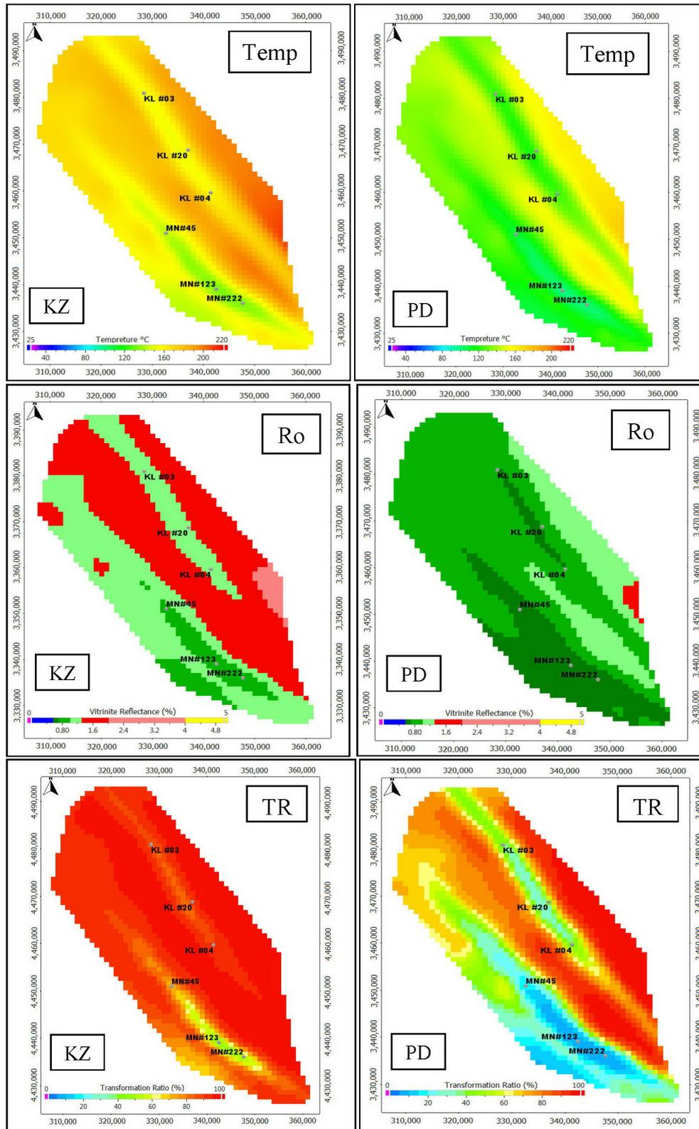
Figure 21. The Vitrinite reflectance, Temperature and Transformation ratio maps of Kazhdumi and Pabdeh source rocks at Present day in drainage area between Kupal and Marun oil fields.
