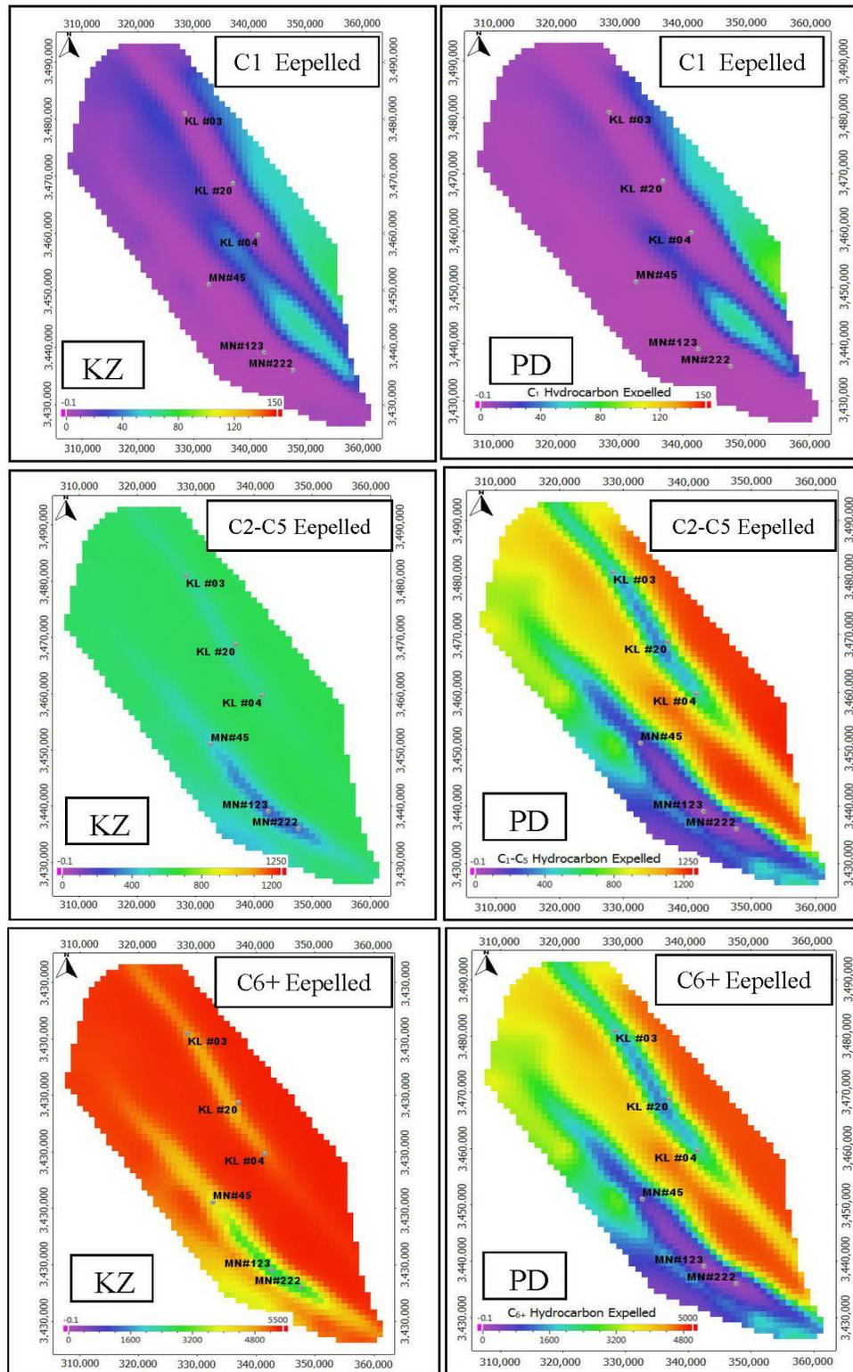
Figure 18. The hydrocarbon compounds expelled from Kazhdumi and Pabdeh source rocks in drainage area of Marun and Kupal oil fields.
