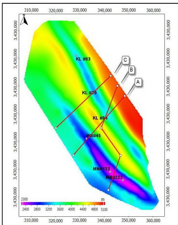
Figure 15. Position of selected cross axial profiles of A, B and C on the Asmari horizon of the Kupal and Marun fields.
