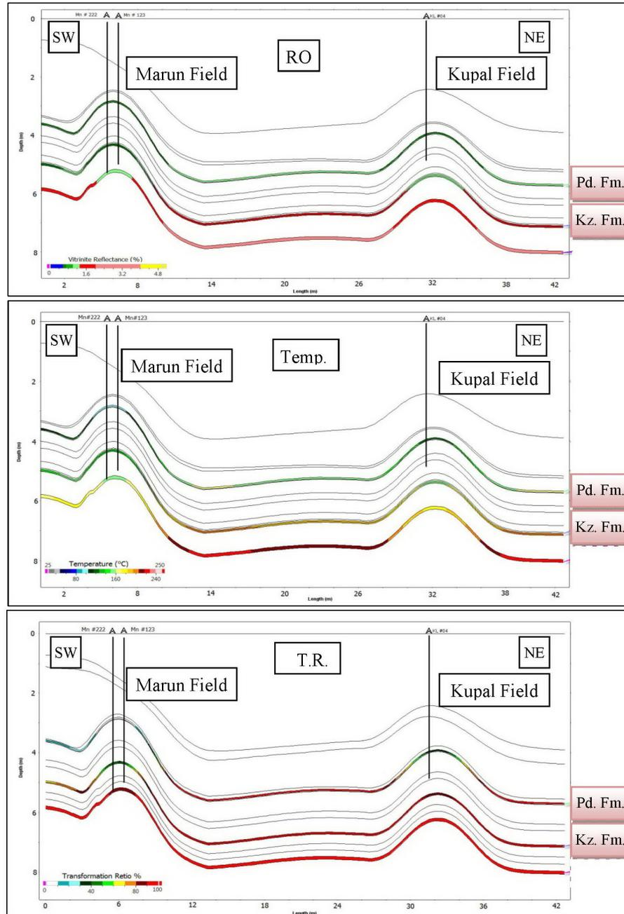
Figure 20. The Vitrinite reflectance, Temperature and Transformation ratio Values of the Kazhdumi and Pabdeh source rocks on Profile (B) at Present day in drainage area between Kupal and Marun oil fields.
