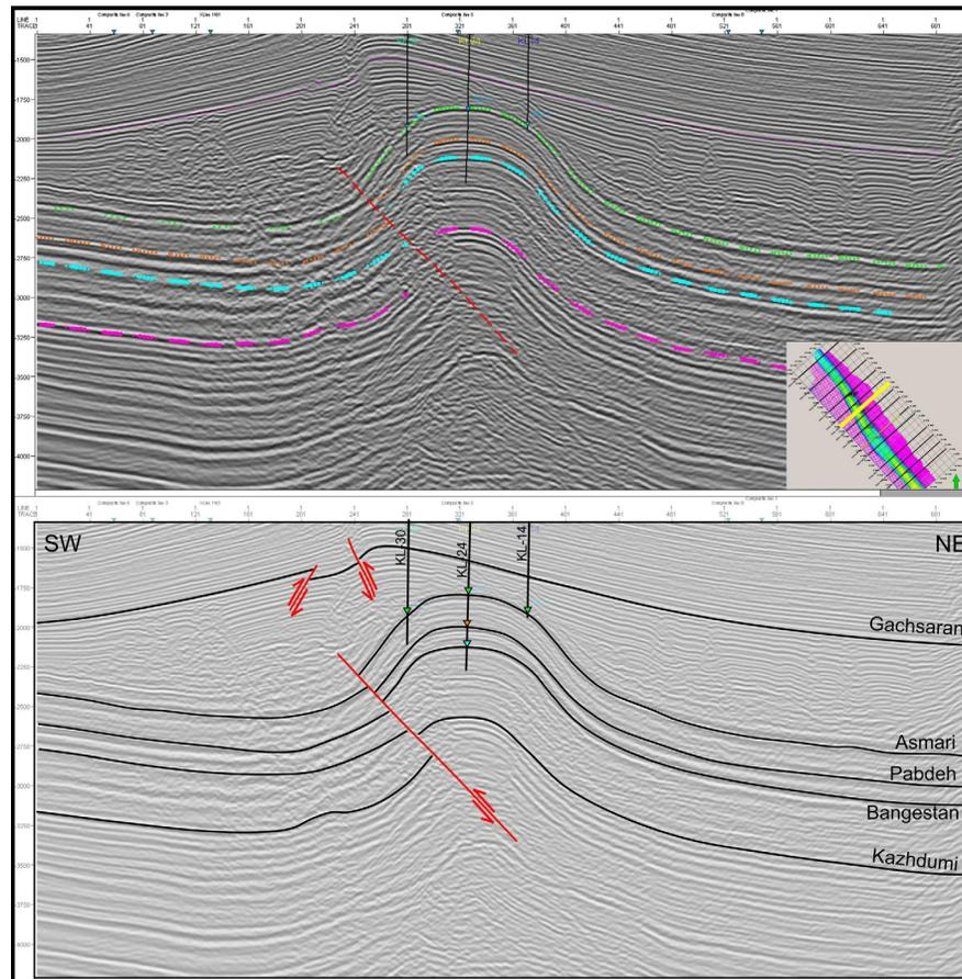
Figure 4. Seismic cross-axial profile in the western culmination of Kupal anticline which passes through wells no. 14, 24, and 30
