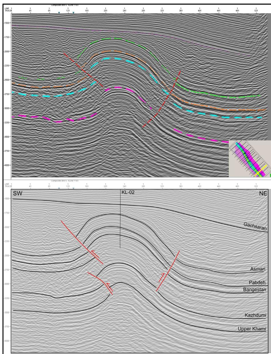
Figure 5. Seismic cross-axial profile in the eastern culmination of Kupal anticline which passes through Well no.2
