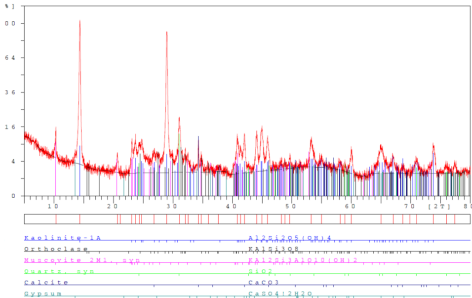
Figure 5. XRD analysis of Kaolinite.
