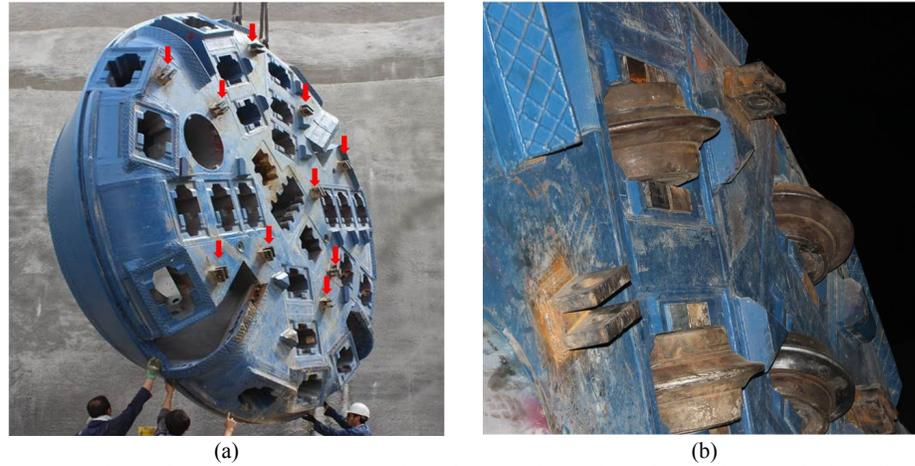
Figure 10. a) The position of new rippers on the cutterhead face; b) Closer view of welded blocks for installing new rippers
