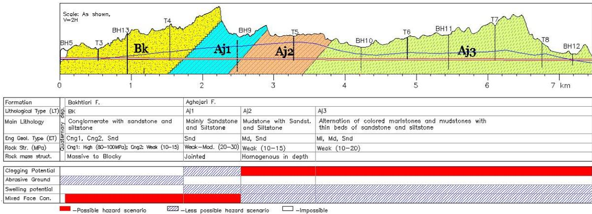
Figure 3. Geological profile of the tunnel and geological problems identified along the tunnel.
