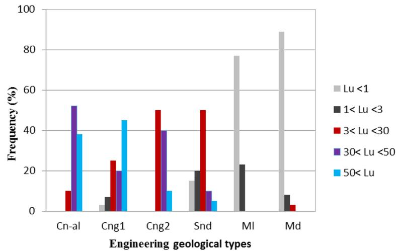
Figure 5. Variations of Lugeon values for various engineering geological types
