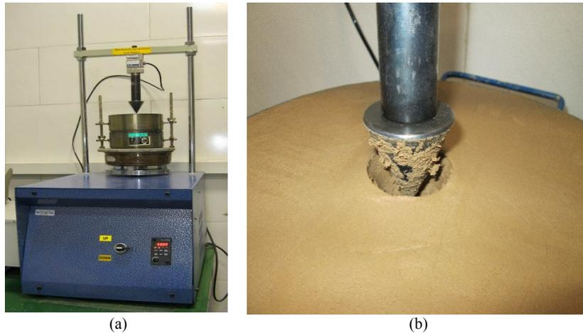
Figure 8. a) Cone pull-out apparatus at the University of Tehran and b) a picture of a sample during test
