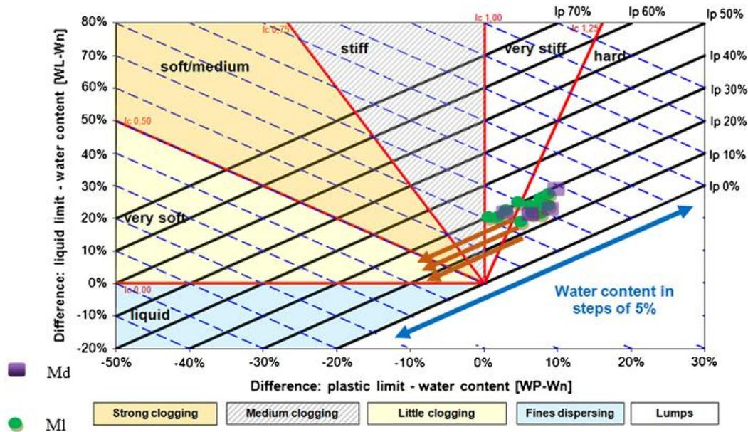
Figure 7. Classification diagram for critical consistency changes regarding clogging and dispersing (Hollman & Thewes, 2013) with samples from the CWCT project.
