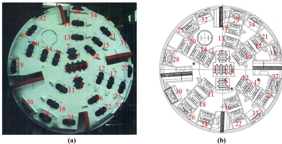
Figure 2. Picture (a) and drawing (b) of the original cutterhead (the numbers indicate cutter positions in cutterhead)
