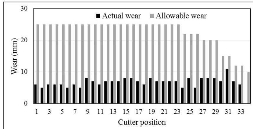
Figure 11. Actual wear of disc cutters in excavated length of tunnel (about 1500m)
