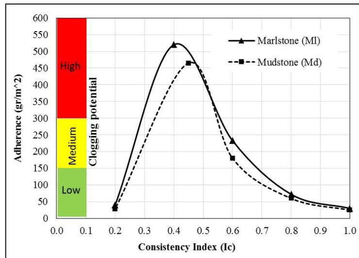
Figure 9. Variations of Adherence with consistency index of tested materials
