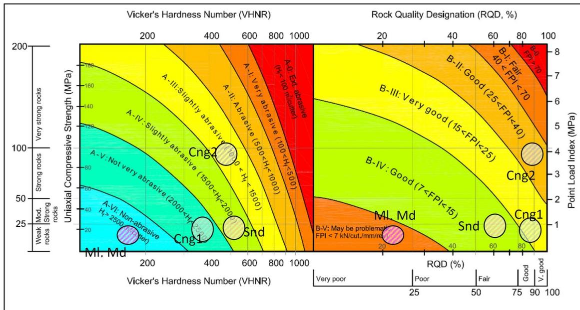
Figure 6. General cutter life and boreability prediction chart (Hassanpour *et al.*, 2015) and range of boreability and abrasivity of engineering geological types in the CWCT project
