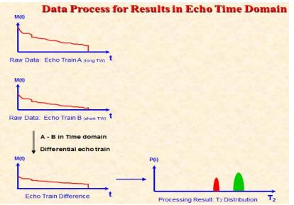
Figure 1. Hydrocarbon typing using TDA technique
