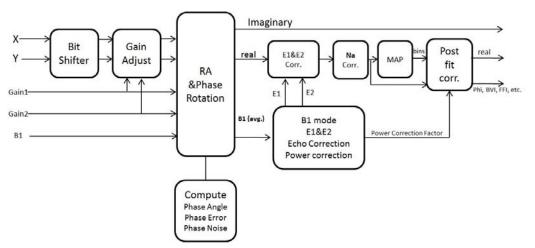
Figure 4. Signal processing steps(Coates et al., 1999)
