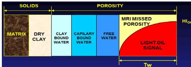
Figure 7. Schematic of hydrocarbon correction by using TDA technique
