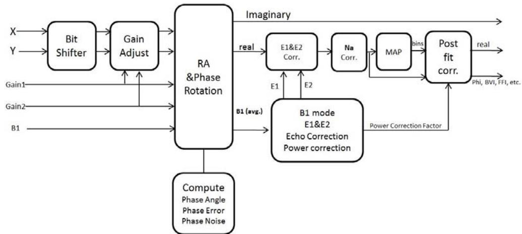
Figure 4. Signal processing steps(Coates *et al.*, 1999)
