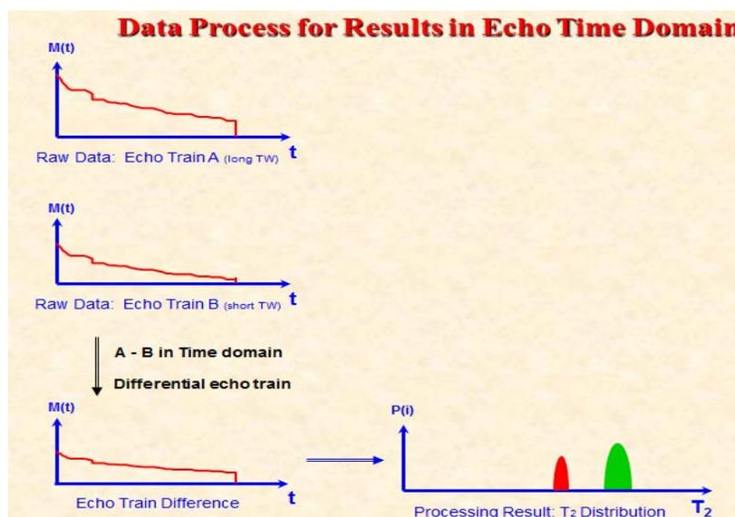
Figure 1. Hydrocarbon typing using TDA technique
