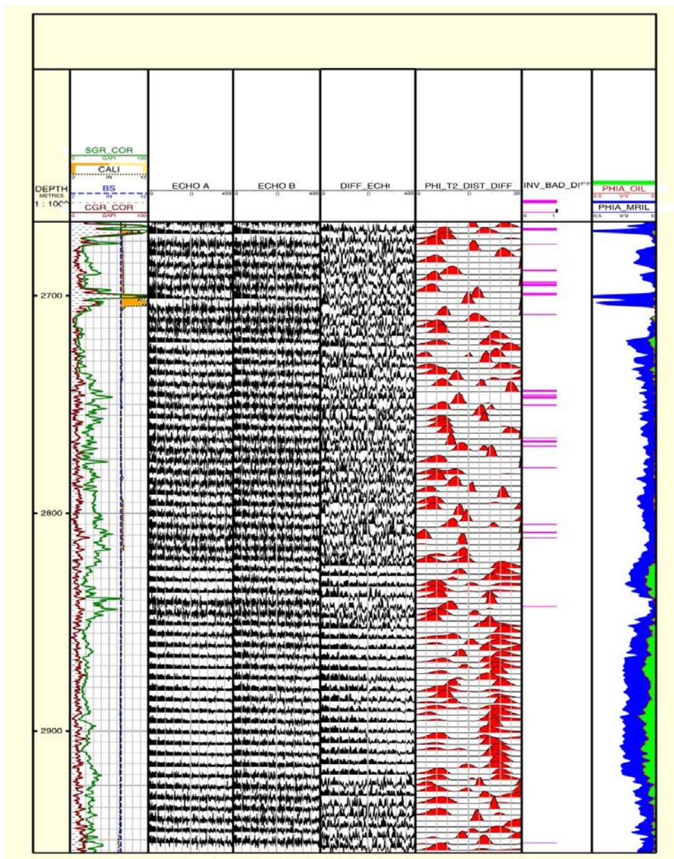
Figure 8. Calculated volume of oil and water by TDA technique
