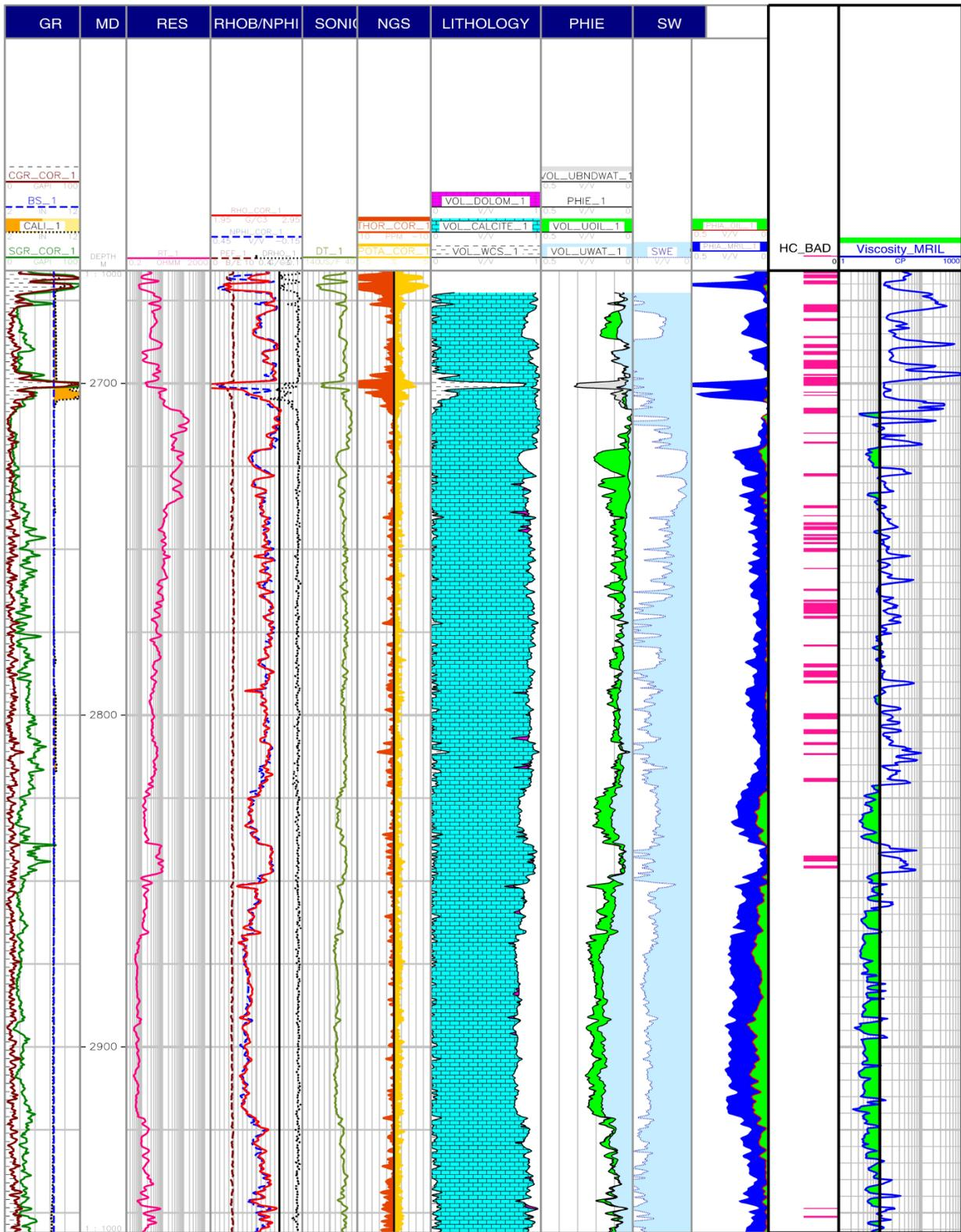
Figure 9. Comparison between hydrocarbon volumes obtained from conventional (FULLSET) logging and TDA. Calculated values of viscosity are indicated in the last Column.
