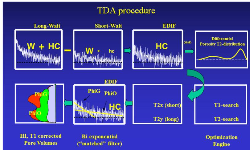
Figure 6. Step of process TDA technique
