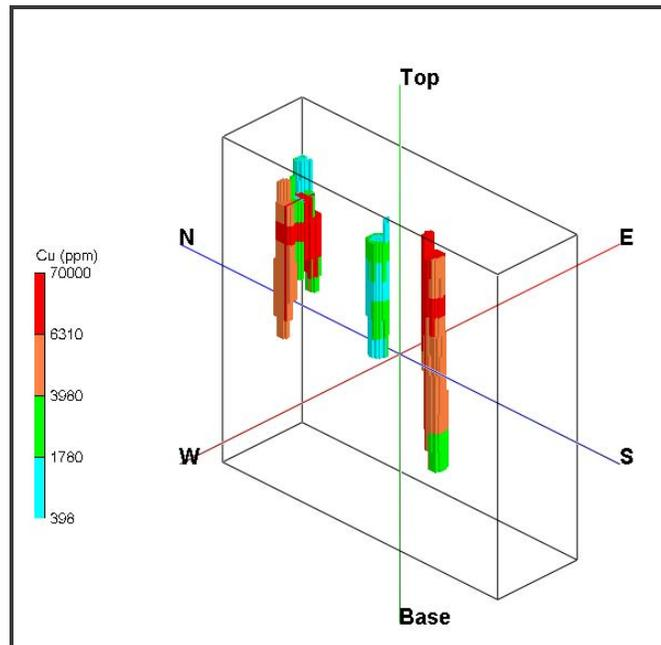
Figure 6. 3D model for Cu distribution
