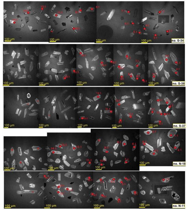
Figure 3 Cathodoluminescence (CL) images of zircon grains selected from a number of post-ophiolite adakitic samples. Targeted SHRIMP U–Pb analytical spots are indicated on the figures as solid circles.
