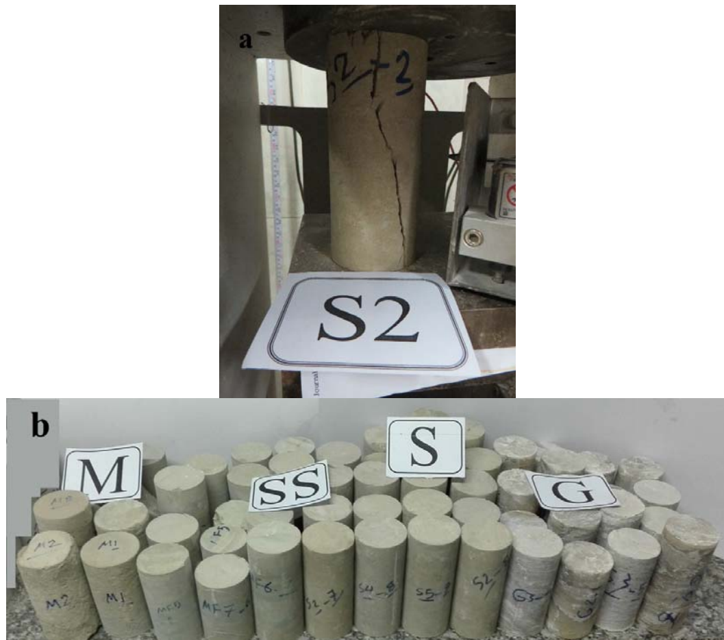
Figure 4. a: The uniaxial compressive strength test setup, b: some of core samples used for laboratory tests.
