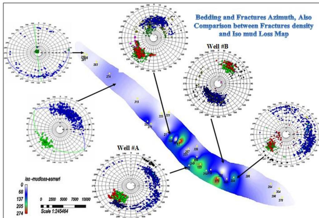
Figure 5. Represent of stereonet for fractures (blue points) and bedding (green points) on Iso-mud loss map in the studied field. (Mud loss data represents center and eastern as fractured section in the studied field which show high correlation with images data)
