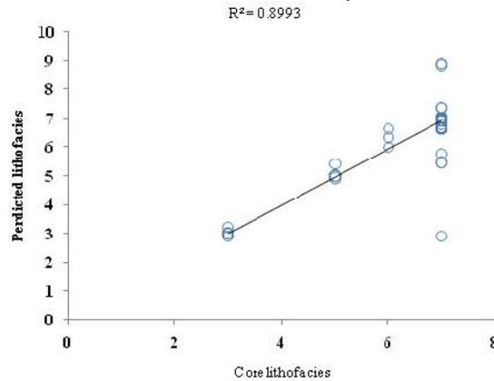
Figure 14. Cross plot of core lithofacies of well# 123 of the Marun oil field and predicted lithofacies from the ANN validation
