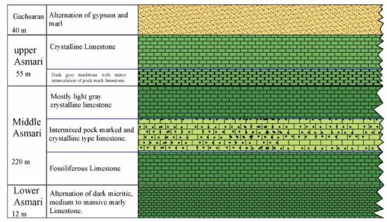
Figure 2. Geological profile around the anticline axis
