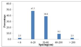
Figure 8. Joint spacing conditions in the right abutment
