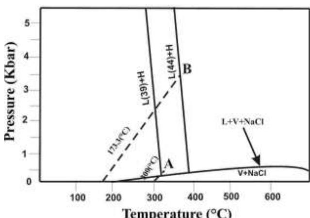
Figure 11: Temperature-pressure diagram of part of the NaCl-H<sub>2</sub>O system (Bodnar, 1994). The dashed lines represent constant liquid-vapor homogenization temperatures which
