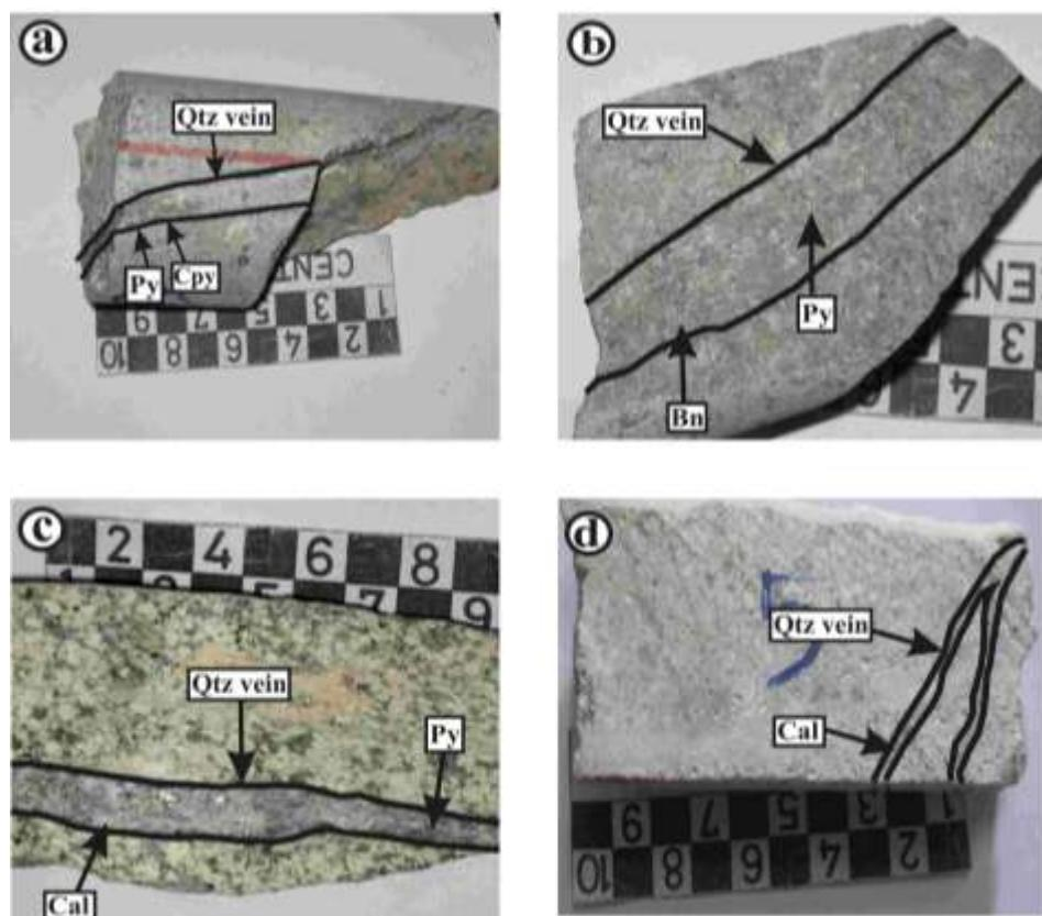
Figure 8. Classification of quartz veins in Sar-Kuh porphyry copper deposit. (a) Group I quartz (Qtz) vein with pyrite (Py) and chalcopyrite (Cpy) grains, (b) Group II quartz vein with pyrite and bornite (Bn), (c) Group III quartz vein with pyrite and calcite (Cal), (d) Group IV quartz vein with calcite.
