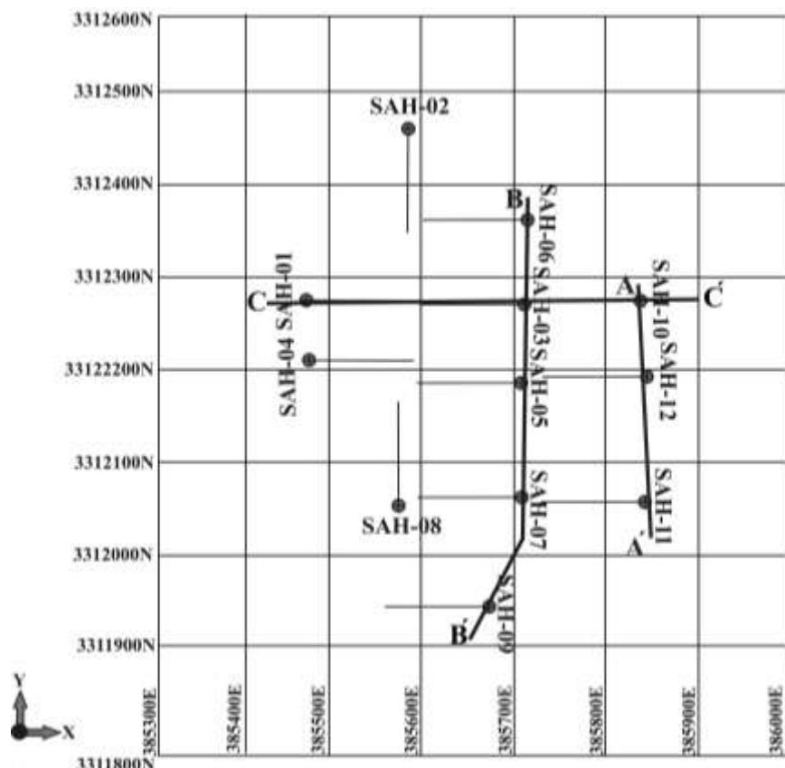
Figure 5: The position of exploration drill holes in Sar-Kuh area. Two cross-sections (A-A' and B-B') were selected to investigate the variation of Cu concentration with depth and alteration type (see figure 4).
