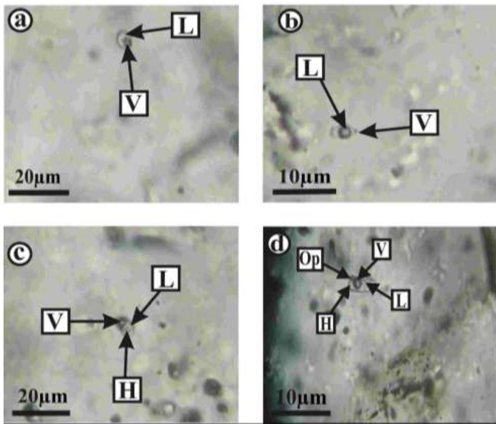
Figure 9: Photomicrograph of fluid inclusions from mineralized quartz veins at Sar-Kuh porphyry copper deposits. (a) LV (liquid+vapor), (b) VL (vapor + liquid), (c) LV associated with halite (liquid+vapor+halite), (d) LVHS (liquid + vapor + halite + solid).
