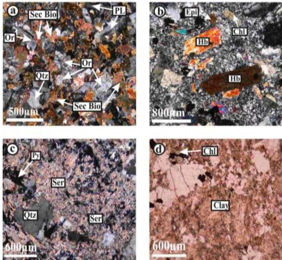
Figure 7: Photomicrograph of (a) potassic alteration, (b) propylitic alteration, (c) argillic alteration, (d) phyllitic alteration that affected Mamzar batholith in Sar-Kuh area. Plain polarized light. Or = Orthoclase, Qtz = Quartz, Sec Bio = Secondary Biotite, Epi = Epidote, Chl = Chlorite, Hb = Hornblende, Py = Pyrite.
