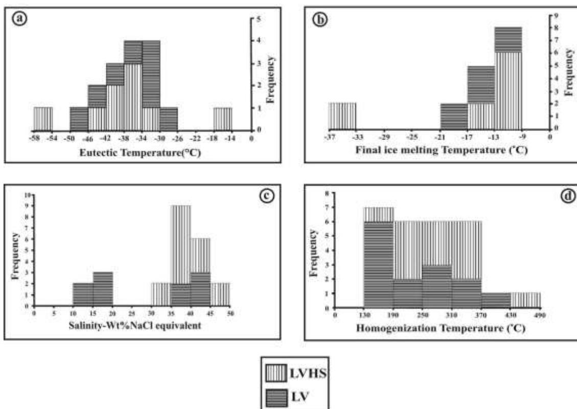
Figure 10: Histograms for LV and LVHS fluid inclusions from mineralized quartz veins at Sar-Kuh deposit. (a) Eutectic temperature, (b) Final ice melting temperature, (c) Salinity, (d) Homogenization temperature.
