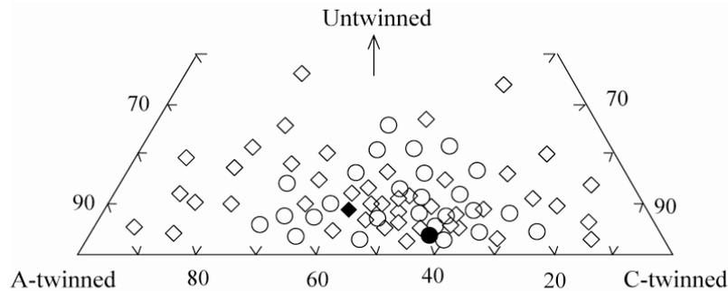
Figure 8: Distribution of major twin types in detrital feldspars of the ZF (circles) and URF facies (rhomboids). The solid circles and rhomboids represent mean values for each formation. Each point represents mean values of 1-10 thin sections.
