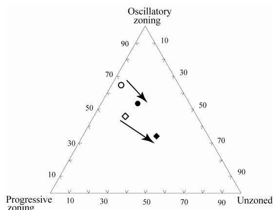
Figure 10: Differences in the average abundance of zoning types in detrital grains of the ZF (solid circle) and the URF (solid rhomboid) facies in comparison to their proposed sources (open circle and rhomboid respectively). The arrows show variation trend of the feldspars during transportation.
