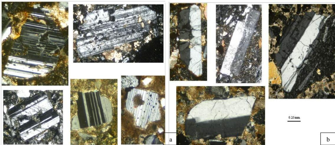
Figure 7: Representative photomicrographs of the A-twinned (a) and C-Twinned (b) feldspars in the facies of studied formations. All figures are in XPL.
