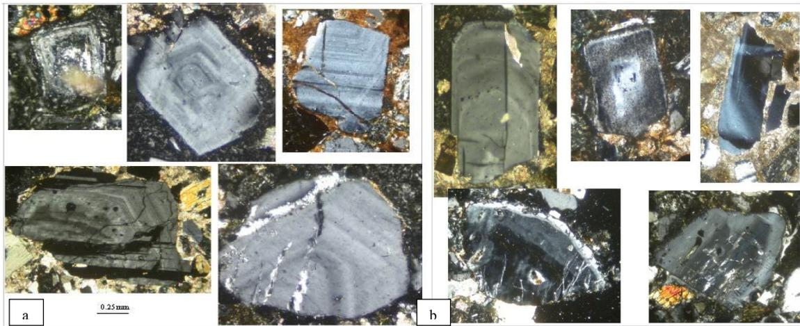
Figure 5: Representative photomicrographs of the oscillatory zoned (a) and progressive zoned (b) feldspars in the facies of studied formations. All figures are in XPL.
