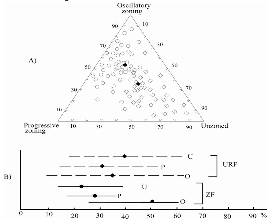
Figure 6: A: Distribution of zoning types in detrital feldspars of the ZF (open circles) and the URF (open rhomboids) facies. Each point represents mean values of 1-10 thin sections. Solid circles and rhomboids represent the mean values for each group. B: Range in abundance of oscillatory (O), progressive (P), and unzoned (U) feldspars and mean value for each group (solid circles and rhomboids).
