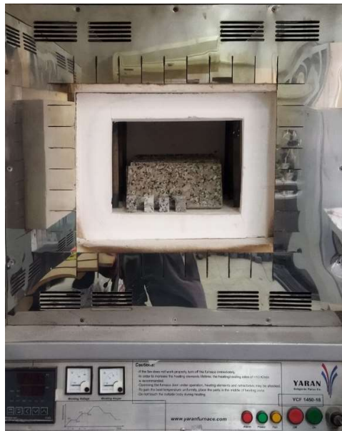
Figure 2. The furnace used in the experiment, equipped with a HANYOUNG controller, model PX
