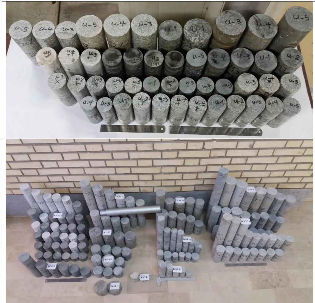
Figure 2. The picture of cylindrical cores rock samples
