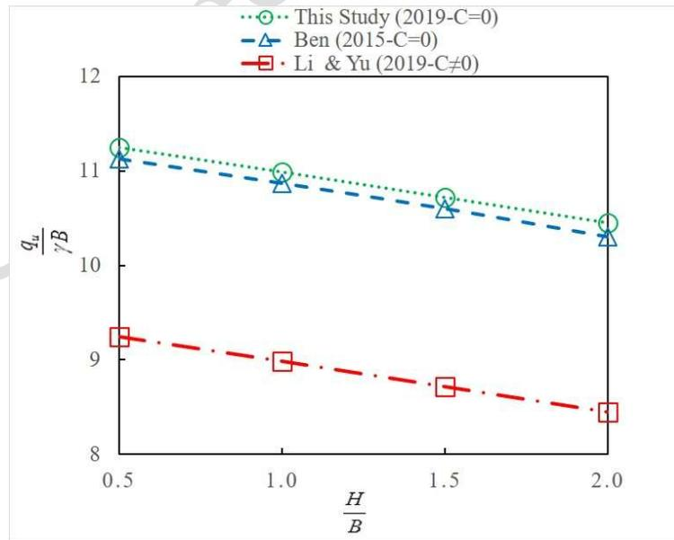
**Figure 12.** Comparison of the present study with other researchers in different positions of the height of slope relative to the foundation width ( $H/B$ ) in the inclined land on cohesive and non-cohesive soils in for:  $\phi = 40^\circ$ ,  $\beta = 45^\circ$ ,  $B = 2$
