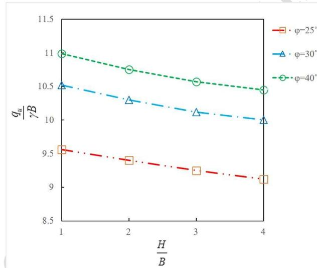
**Figure 8.** Changes in normalized bearing capacity to relative the height of slope to the width of foundation ( $H/B$ ) for:  $\lambda = 0, D \neq 0, B = 2$
