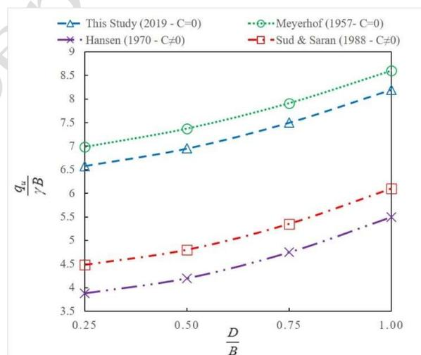
**Figure 10.** Comparison of the present study with other researchers in different positions of embedded Depth relative to the width of foundation ( $D/B$ ) in the inclined land on cohesive and non-cohesive soils in for:  $\phi = 40^\circ, \beta = 45^\circ, B = 2$
