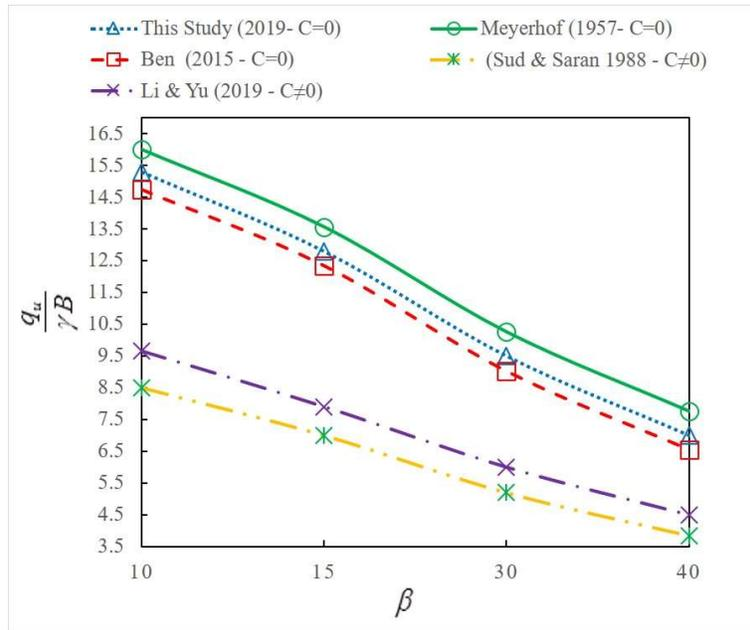
**Figure 11.** Comparison of the present study with other researchers in different positions of slope angle ( $\beta$ ) of foundation in the inclined land on cohesive and non-cohesive soils in for:  $\phi = 30^\circ$ ,  $\beta = 45^\circ$ ,  $B = 2$
